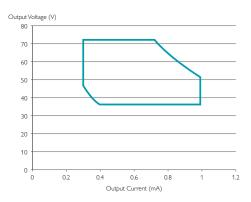
Example of operating window of FlexDrive/TD or Rset driver. Can operate all points within window
