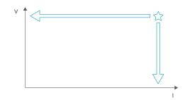
Example of peak design driver fixed output driver with fixed current and voltage setting (only drives a module with specs at star (in reality a small operation line)
